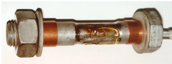
Fig. 3: Bolt M30 with strain gauges
